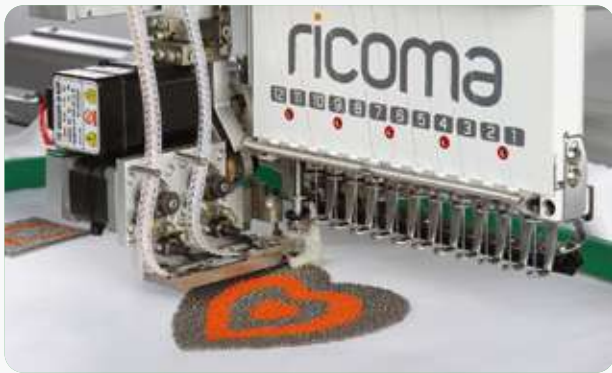
Bead Device Explore your creativity to include intricate bead work with the optional bead device.
