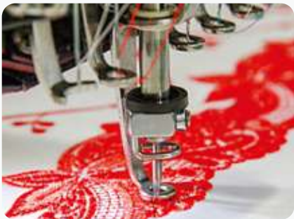
Boring Needle This specifically designed needle creates intricate embroidery by piercing the fabric, cutting it into various shapes, and leaving holes in the item.
